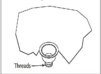
3. Attach a 3/4" drainage hose (not included) to the blue hose fitting.
