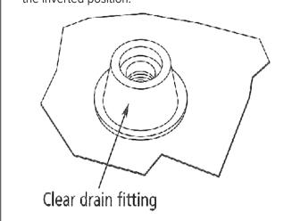
2. From the bottom side of the unit, insert a finger into the center of the clear drain fitting. Pull outward on the inside of the fitting to reveal the external threads.
