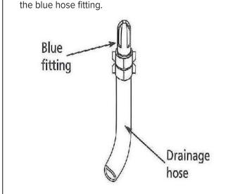
4. Attach the hose assembly (blue fitting and 3/4" drainage hose) to the clear drain fitting on the unit.
