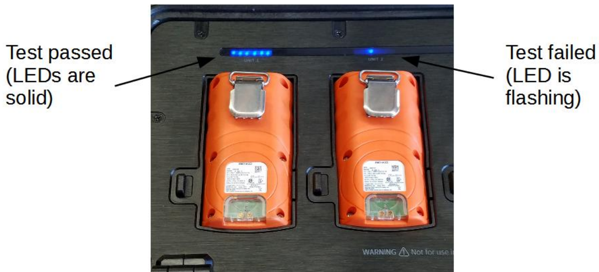
Figure 4–1 LED pattern indicates test pass or fail
