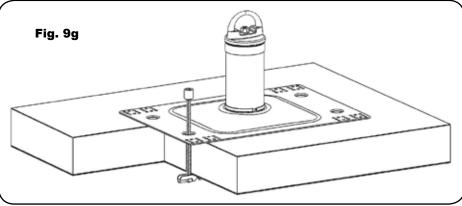
11. Once toggle is fully drawn up and seated (see Fig. 9h and 9i), torque to approximately 10-15 ft lbs. Repeat for other three toggle bolt assemblies.
