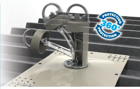
In the event of a fall, the Miller Fusion Roof Anchor Post orients in the direction of the force, the built-in, energy-absorbing component activates and the base remains securely attached to the roof surface.
