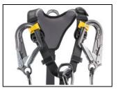
The MGO connectors on fall arrest lanyards can be stowed on each shoulder strap. The user is thus unhindered by the lanyard, and the connectors stay within reach. In case of a fall, this system releases the MGOs and allows the absorber to be deployed.
