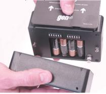
To reinstall the source module onto the base module, take the following steps: Align the air inlet fitting and the locking pins into the eyelet holes as shown. Press the two units together and slide the source module upwards (relative to the base module) to lock it in place. The two units should be flush and tightly secured at this point, then simply slide the base plate back into position until it latches.
