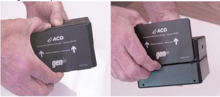
With the base plate out of the way it is now possible to disengage the source module. This is accomplished by sliding the source module downward (relative to the base unit) as shown.
