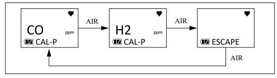
8. Press and release POWER MODE. The calibration value begins to flash.
