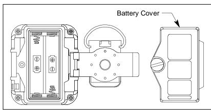
Figure 9: Battery Cover Removal
