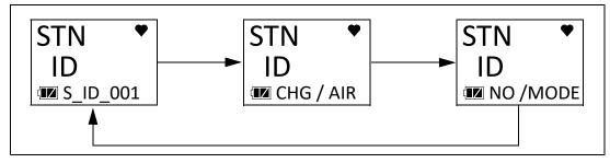
2. To change the Station ID, press and release AIR. The current Station ID flashes.
