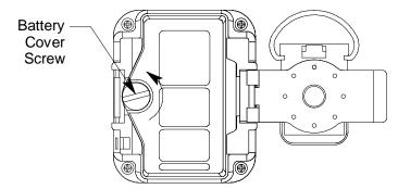
Figure 8: Unscrew Battery Cover Screw
