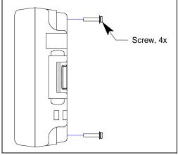
Figure 14: Unscrewing Case Screws
