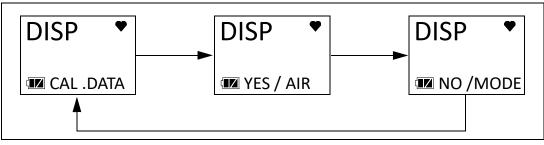
2. Press AIR to enter the CAL.DATA screen. The date of the last successful calibration displays.
