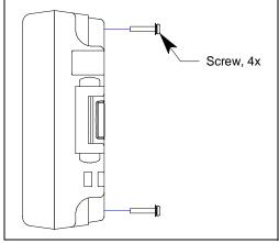
Figure 17: Unscrewing Case Screws
