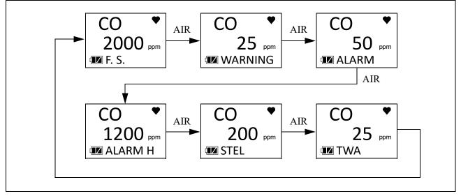
4. Press and release POWER MODE to return to the Alarm Points Screen.
