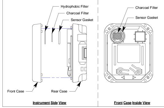
**Figure 16: Hydrophobic Filter Location**
