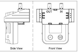
4. Use the tubing to connect the regulator to the inlet of the calibration cup (labeled "IN").
