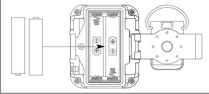
**Figure 10: Installing New Batteries**
