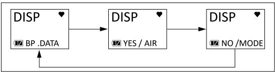
2. Press AIR to enter the **BP.DATA** screen. The date of the last successful bump test displays.
