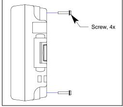
Figure 11: Unscrewing Case Screws
