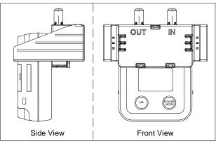
3. Use the tubing to connect the regulator to the inlet of the calibration cup (labeled "IN").
