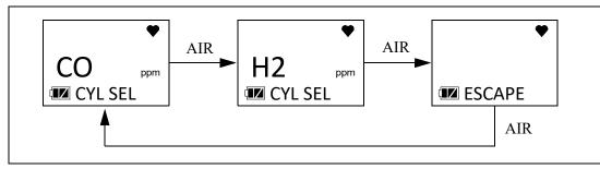
8. Press and release POWER MODE. The current setting flashes. In the example below, CO is selected.
