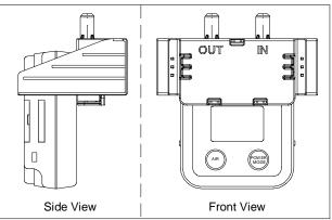
4. Use the tubing to connect the regulator to the inlet of the calibration cup (labeled "IN"). *Performing a Calibration*
