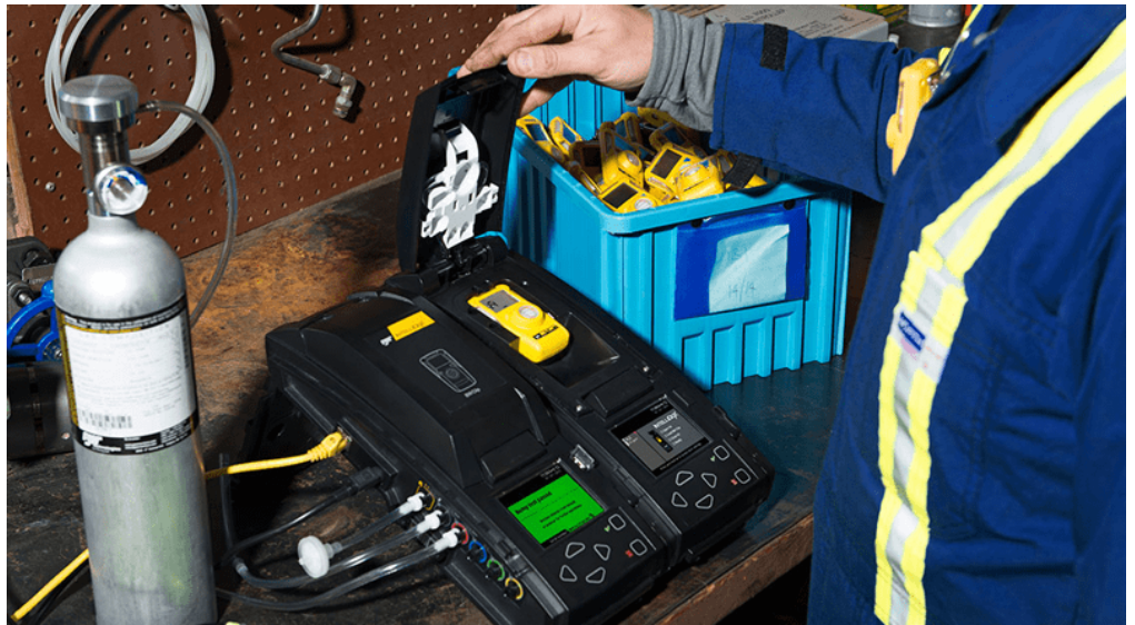
A docking station is used to automatically calibrate gas monitors and update calibration records.
