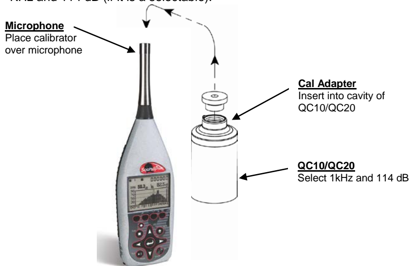
Figure 5-2: Attaching calibrator to SoundPro
